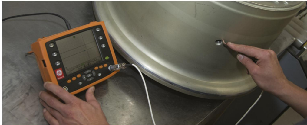
NDT testing is important to detect damage, but some operators only send wheels for repair when the damage is visible (photo: World Aero)
